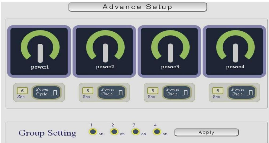
For example : The following pictures means that Power #1 & #4 is ON , Power #2 & #3 is OFF
