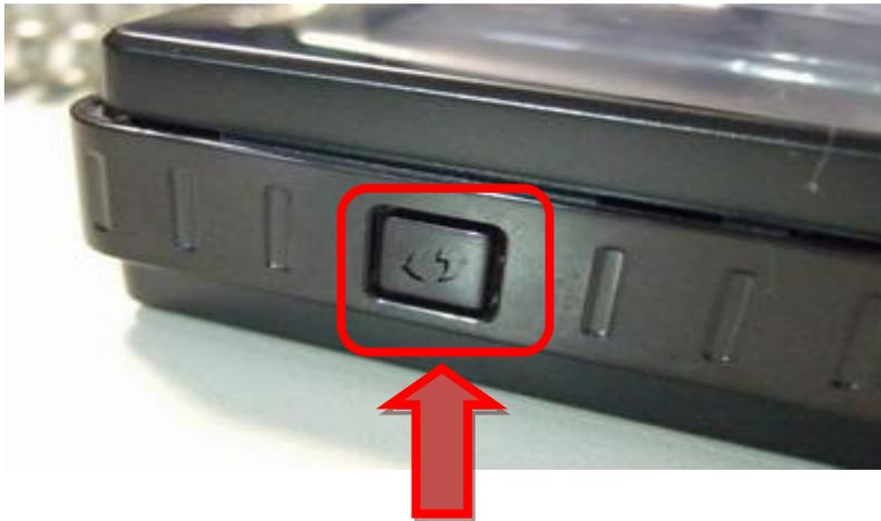
Step 3 : Press One time ( short ) the " Reset button" of 9258W2 and then there is one long beep which means the WPS function of 9258W2 enable .
